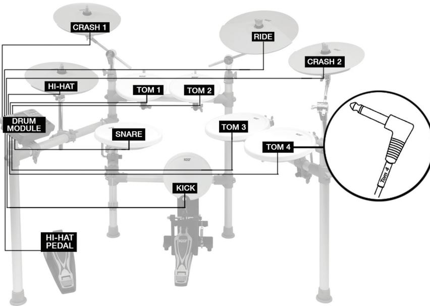
1. Place the Kick on the floor, in the center of the rack as shown below.
