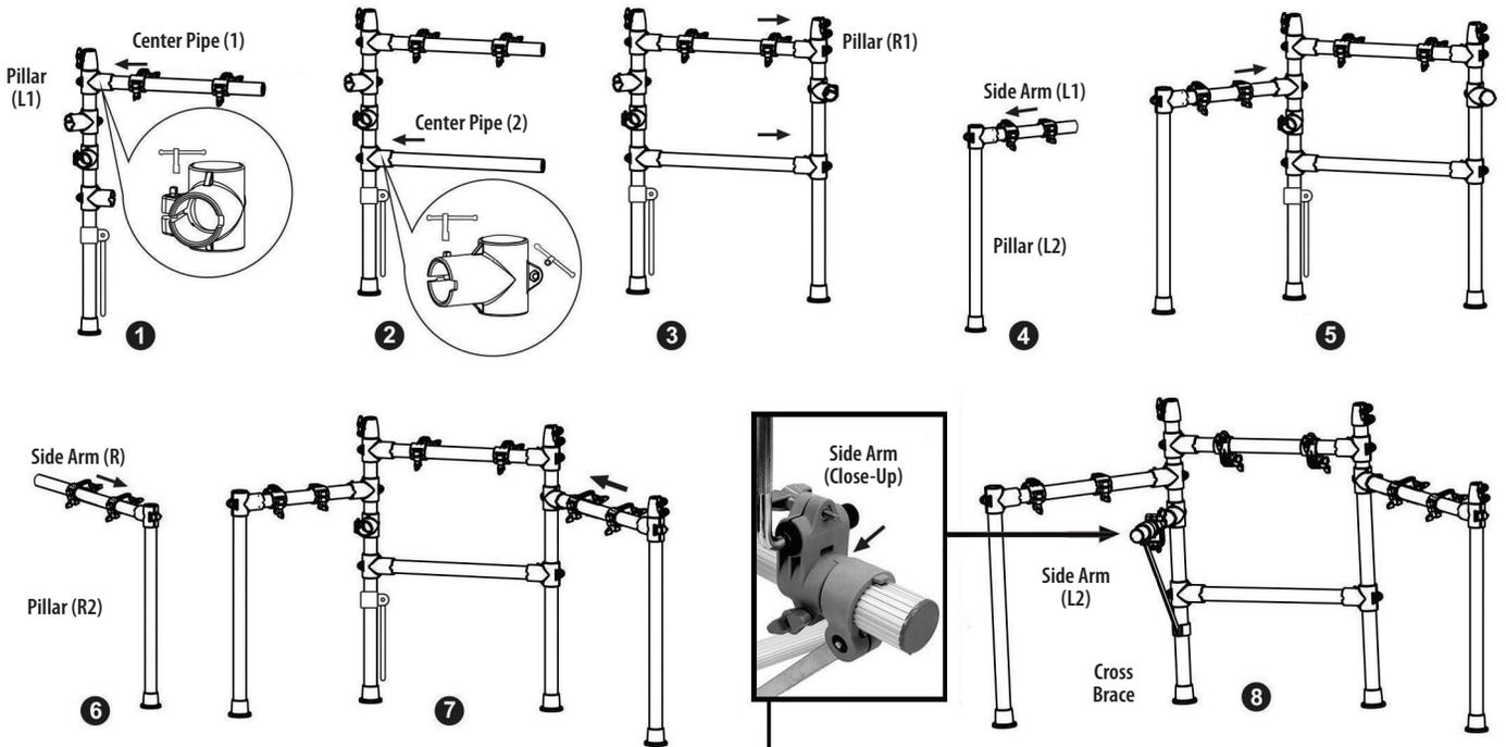
1. Attach Center Pipe (1) to clamp on Pillar (L1).
