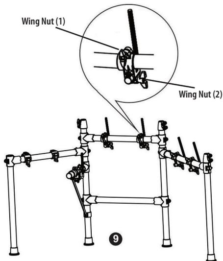
9. Attach the pad mounts to the mount holders on the Center Pipe 1, Side Arm (L2), Side Arm (R), and firmly tighten the respective wing nuts 1.
